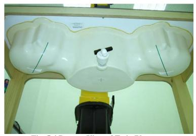
Fig. 5.4 Bottom View of Twin Phantom
