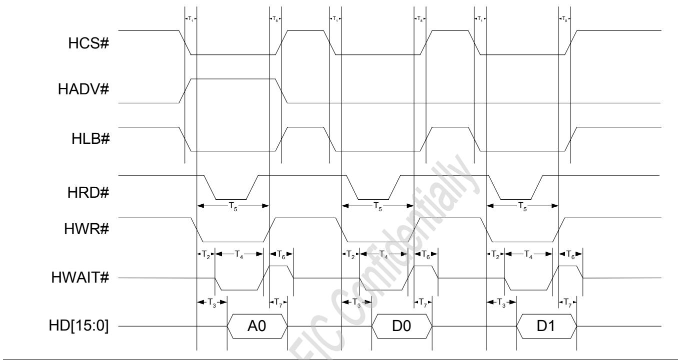
Figure 3.1.6-3 Indirect Addressing Mode 16 bits 68 Type Read Transaction
