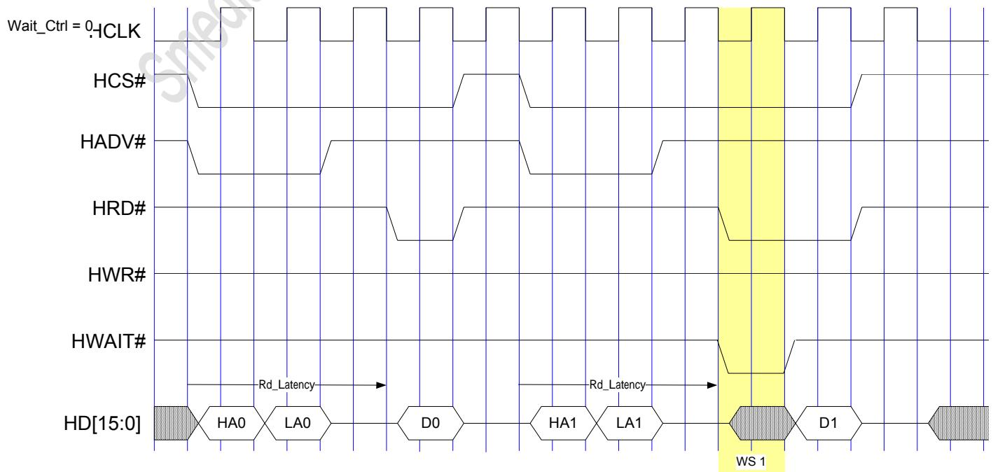
Figure 3.1.9-8 iBurst Burst Read Transaction with Wait\_Ctrl =1 (High-Low Addressing Multiplex)
