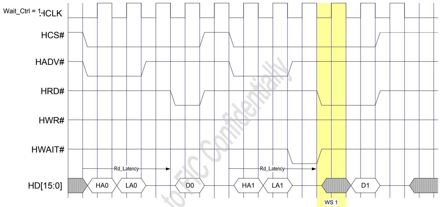
**Figure 3.1.9-7 iBurst Single Read Transaction with Wait\_Ctrl =0 (High-Low Addressing Multiplex)**
