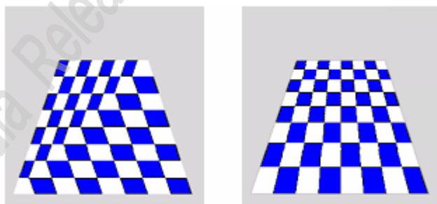
Example of without perspective correction and with perspective correction
