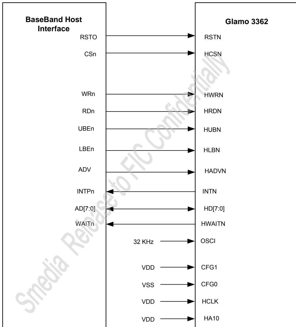
**Figure 3.1.8-2 Indirect Addressing Mode 8 bits 68 Type Write Transaction**
