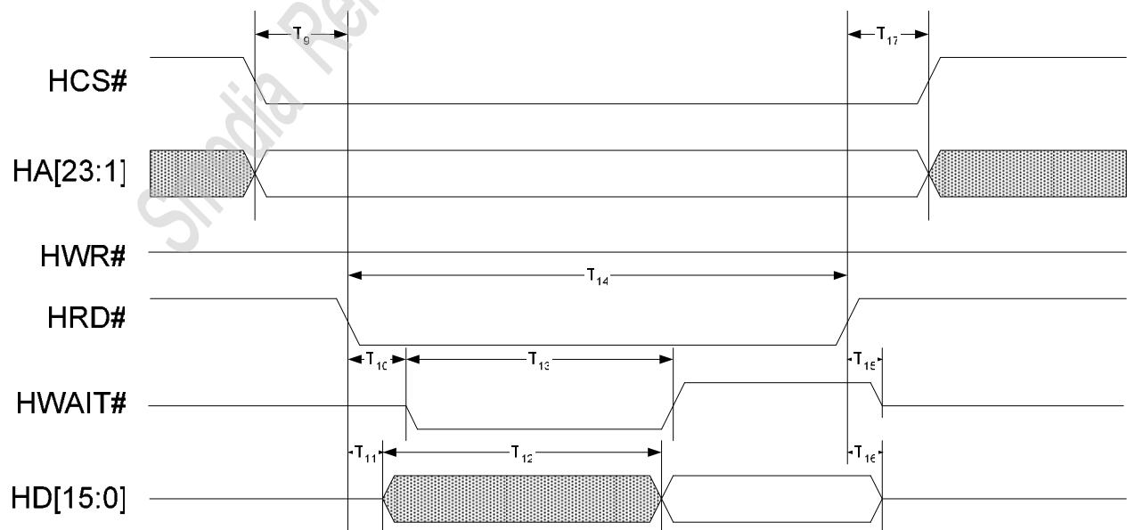
**Table 3.1.3-1 Direct Addressing Mode 16 bits 80 Type 2 Interface Timing Table**
