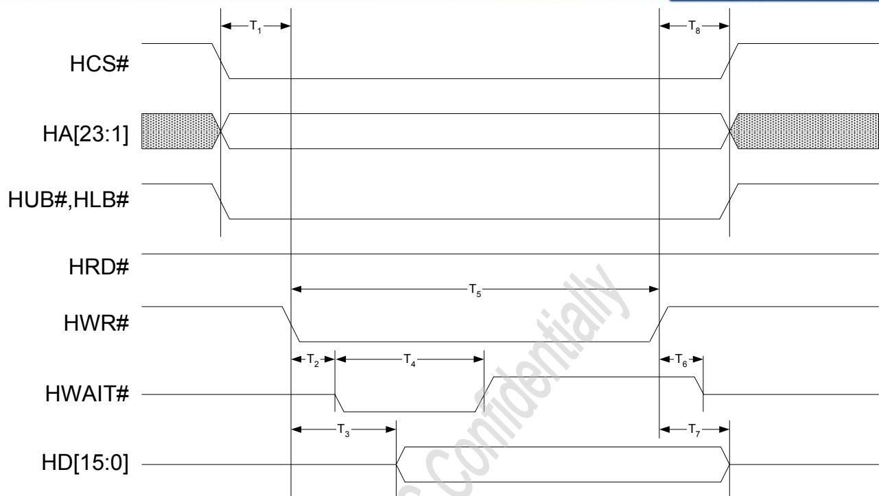
Figure 3.1.2-3 16 bits 80 Type 1 CPU Read Transaction
