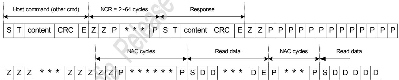
**Figure 3.4.2-4 MMC/SD Single Block Write Protocol**
