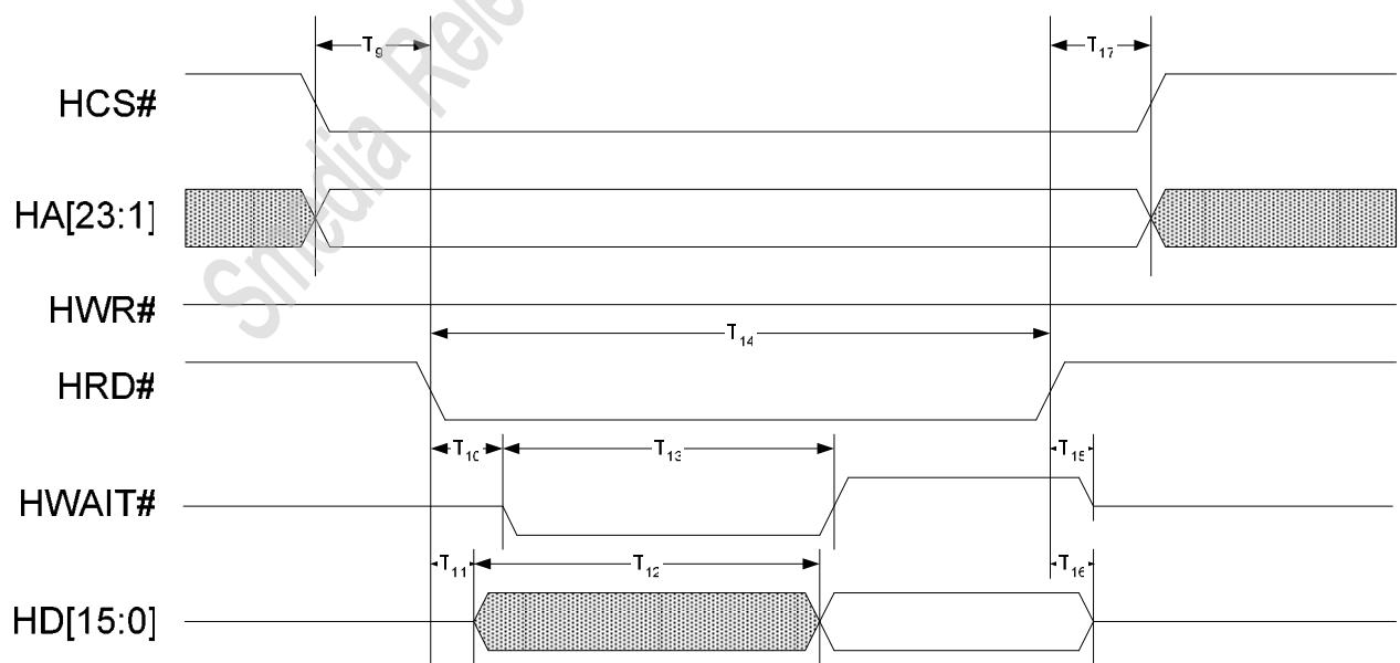
**Table 3.1.4-1 Direct Addressing Mode 16 bits 68 Type Interface Timing Table**
