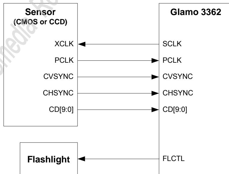
Figure 3.3.2-2 Connection of Glamo 3362 to Sensor (Mode 2)
