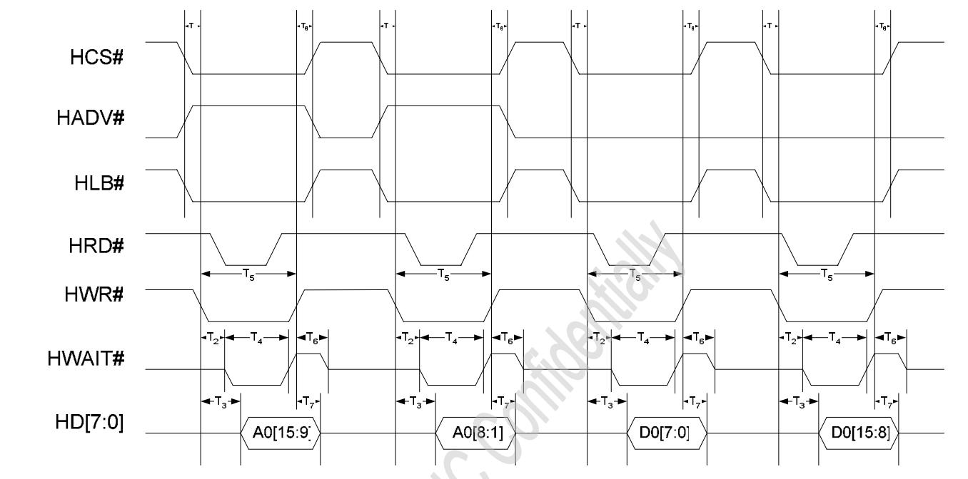
**Figure 3.1.8-3 Indirect Addressing Mode 8 bits 68 Type Read Transaction**
