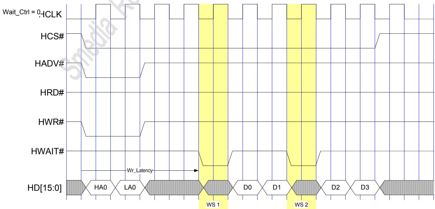
**Figure 3.1.9-6 iBurst Single Read Transaction with Wait\_Ctrl =1 (High-Low Addressing Multiplex)**
