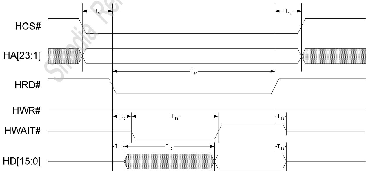
**Table 3.1.2-1 Direct Addressing Mode 16 bits 80 Type 1 Interface Timing Table**
