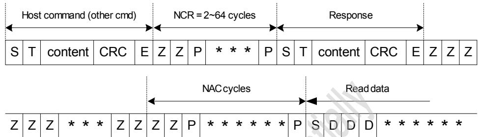
**Figure 3.4.2-3 MMC/SD Multiple Block Read Protocol**
