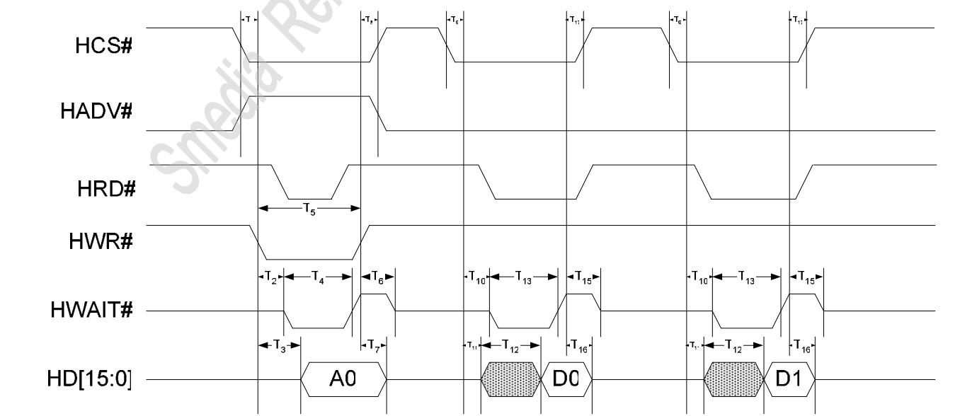
**Table 3.1.6-1 Indirect Addressing Mode 16 bits 68 Type Interface Timing Table**
