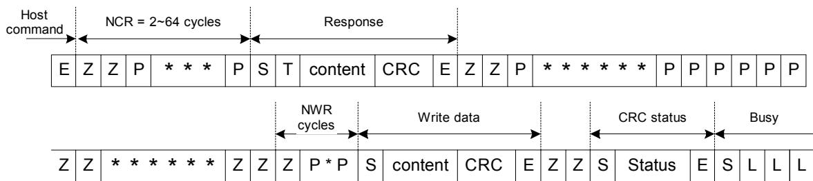
**Figure 3.4.2-5 MMC/SD Multiple Block Write Protocol**
