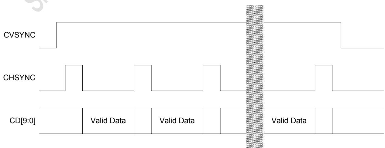
**Figure 3.3.3-3 Video Interface: Negative CVSYNC with Positive CHSYNC**
