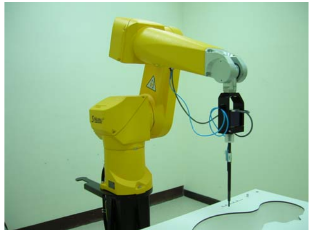
Fig. 5.2 Probe Setup on Robot
