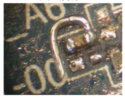
Next I placed the  $100\mu F$  cap and marked where I should scratch off the paint on the motherboard. On these tant caps the +'ve side (anode) has the line, as per the datasheet (see above link\*)
