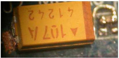
I tinned the pads on the cap, though I'm not sure if this is necesary, I'd recommend only a little.
